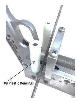
Figure D Horizontal border cut made on the lower edge of the radius of a "non-high" grip frame.
