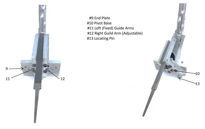
Figure G Setting the file for horizontal serrations – first position. The file should not bind in any position.
