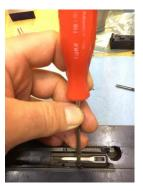
to the screw area as these are retained with a permanent Loctite.
