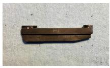
Confirm the firing pin retaining pin is flush on both sides. Install back into the slide. Tap the breech block with a plastic/wood dowel to confirm it has been seated flush in the slide. Make sure the breech block retaining screw and threaded hole in the slide have been cleaned with alcohol. Using a permanent
