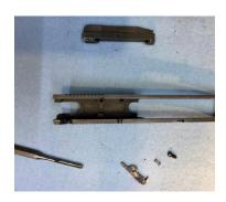
Remove breech block from the slide. A gentle tap may be required to remove the block due to our snug fit. Support breech block on a hard surface and drive the firing pin retaining pin out using a 3/32" punch. Remove firing pin and spring and clean the interior of the breech block.
