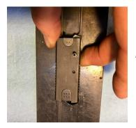
Start extractor roll pin into top of slide. Insert extractor spring and extractor into slide and hold flush to side of slide. Make sure extractor is pulled back onto the breech block face. This will create proper alignment for the roll pin. Drive extractor roll pin just past flush using a 1/8" roll pin punch.
