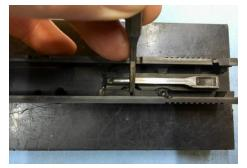
Use a small roll pin punch and remove the extractor roll pin. This MUST be driven from bottom through top or damage to the slide will occur. Remove extractor and spring from slide and set aside.
