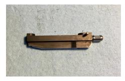
Start the firing pin retaining pin into the breech block. Install the firing pin and firing pin spring. Index the firing pin head notch so as the retaining pin goes in it clears the firing pin without damage. Set on a hard surface and compress the breech block assembly while driving the retaining pin to flush.
